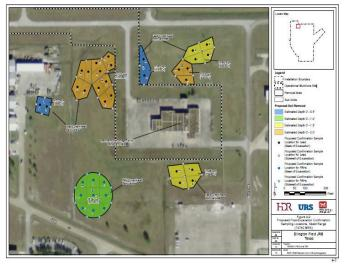
During soil excavation, an X-ray fluorescence (XRF) analyzer was used in the field to determine lead concentrations. Soil above the NTCRA criteria for lead in residential soils (i.e., 358 milligrams per kilogram [mg/kg]) will be excavated and disposed off-site. If XRF results
